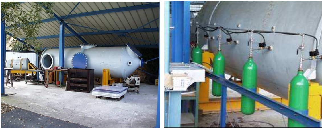
Figure 2 : sketch (dimensions in mm) and views of the 10.5 m 3 chamber (injection device of the fuel on the right picture)
