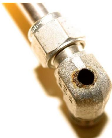
Figure 8. Photograph of a stainless steel fitting drilled by a  $\text{H}_2/\text{O}_2$  flame formed inside the PEM stack.
