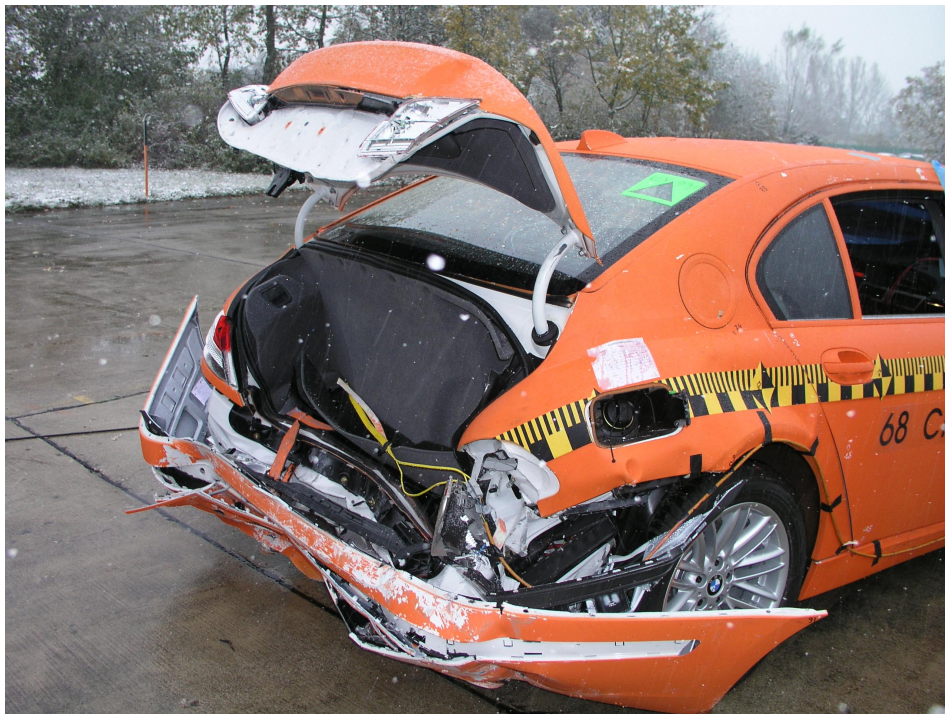
Fig. 3: Offset rear crash according to FMVSS 301
