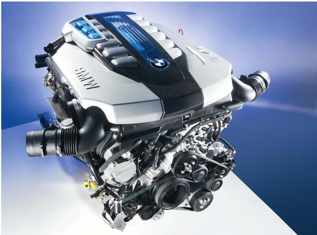
Fig. 5: Hydrogen internal combustion engine
