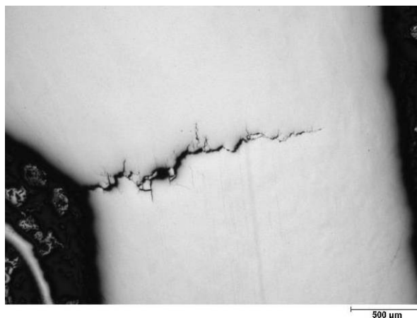
Figure 2. Stress corrosion cracking of stainless steel in potassium hydroxide, water electrolyser
