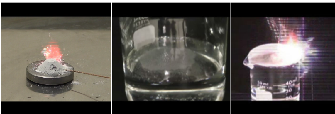
Figure 1. Results from the Water Contact Test for 2\text{LiBH}_4\cdot\text{MgH}_2 . a) Water Drop Test. b) Water Immersion Test, and c) Surface Contact Test.
