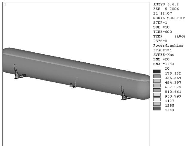
Figure 5: Detailed simulation of the temperature on the shell of a 100 m<sup>3</sup> pressurized vessel under radiation due to flame engulfment (120 kW/m<sup>2</sup>, 600s)
