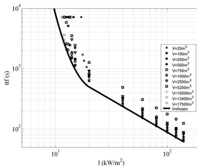
Figure 9: Envelope of times to failure obtained for vertical cylindrical atmospheric vessels under distant source radiation
