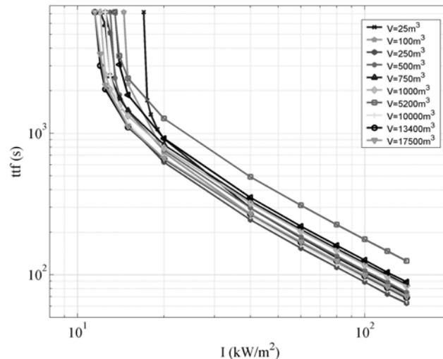
Figure 7: Times to failure obtained for vertical cylindrical atmospheric vessels under distant source radiation
