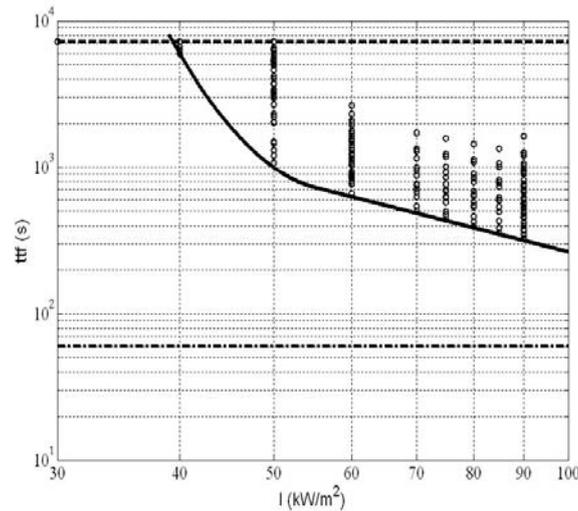
Figure 10: Envelope of times to failure obtained for horizontal cylindrical pressurized vessels (1.5 to 2.5 MPa design pressure) under distant source radiation
