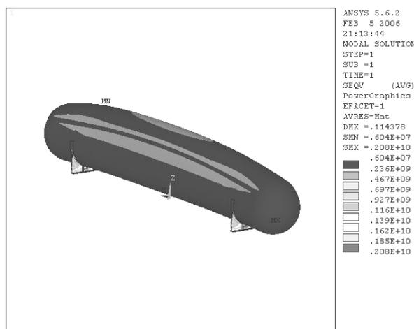
Figure 6: Detailed simulation of the stresses on the shell of the 100 m<sup>3</sup> atmospheric vessel under the conditions shown in figure 5
