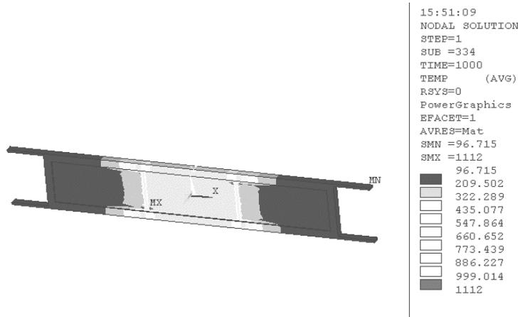
Figure 13. Simulation of the experimental test of a composite protection material under a hydrogen jet flame
