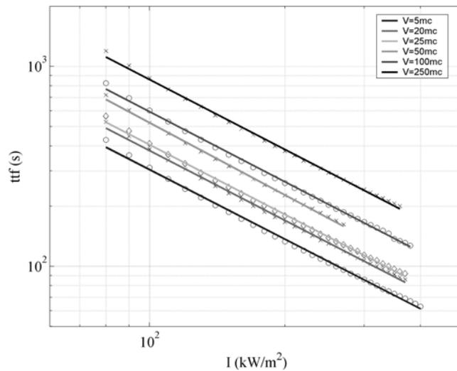
Figure 8: Times to failure obtained for horizontal cylindrical pressurised vessels with length/diameter ratio equal to 1.8. Failure with open PRV under distant source radiation
