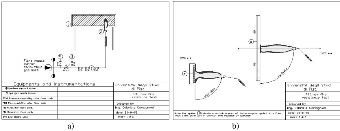
Figure 11. P&I (a) and equipment orientation (b) of the experimental device for the testing of passive protection materials.
