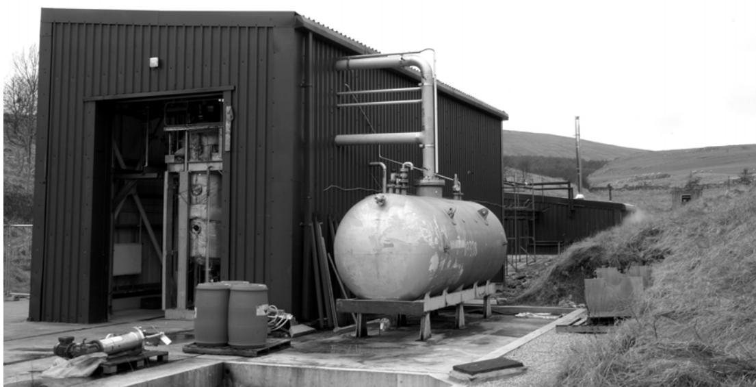
Figure 6. Large-scale facility showing reactor (within building), vent line and external catch tank
