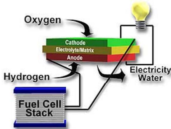
Figure 2 Fuel Cell Configuration US Department of energy, Permitting Stationary fuel Cell Installation, PNNL-14518, 1/12/2004
