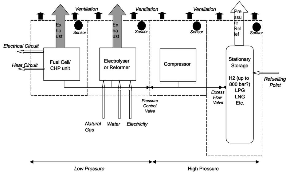
Figure 4 Schematic showing potential elements of stationary fuel cell/hydrogen system. (Note that connections are simply schematic).
